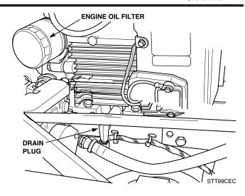
Figure 7-5. Drain Plug Location
